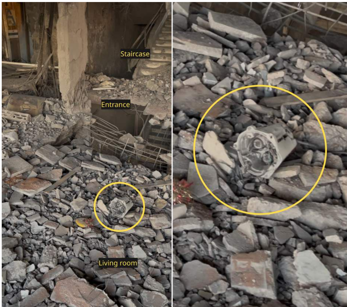
Figure 20: Annotated close-up of the tail actuation system identified in the Cherri flat.
