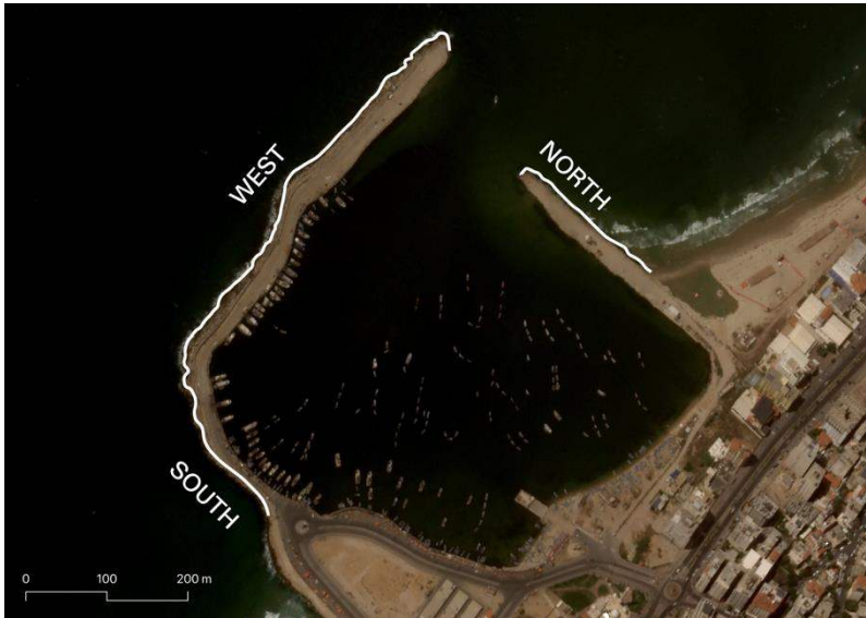
Fig 1. Layout of the port showing the north, the south and the western sections. The marking in white shows the location of the sea wall.
