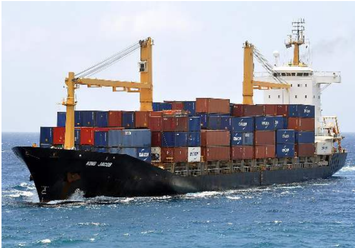
The King Jacob , a 146.42 m-long and 22.7 m-wide cargo ship. Photo credit: Maritime Connector.
