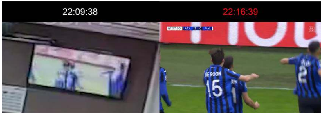
Fig.3: Video B (right) is synchronised with footage from the CCTV system (left), by capturing distinct movements of players after a goal. Above Video B, real time is displayed, as determined by the audio synchronisation with Video A. In the upper left, the time at the same moment according to the CCTV system is displayed. The difference between real time and CCTV footage time is 7 minutes and 1 second.
