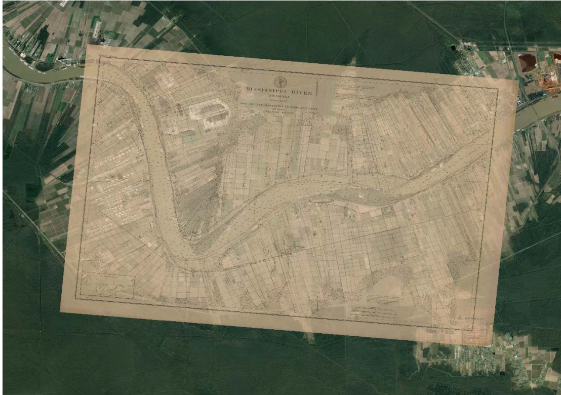
Sheet no. 12, titled "Mississippi River, Louisiana, from Chapman Plantation to Brilliant Point," from the USCS 1878 series, georeferenced within QGIS, and overlaid on top of 2021 Google Earth satellite imagery.
