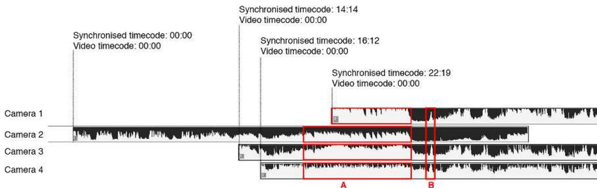
Figure 3. Synchronized audio channels of all four cameras. ‘Synchronised Timecode’ is the time value relative to the synchronization of all 4 videos, ‘Video Timecode’ is the time value relative to the original file.
